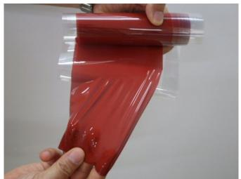
The company says the material combines the best properties of two current piezoelectric (as in able to convert mechanical strain into electrical charge), ceramics and polymers. Ceramics generate "relatively high" electricity but are fragile and heavy, while polymers are flexible but only produce "very slight" power.
