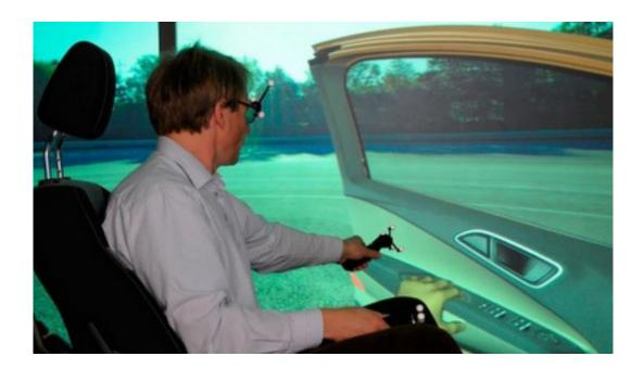
Rather than building expensive prototypes of new cars, Ford uses a **3-D CAVE** for exploring the possible details of new car.
