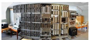
Built in 1951, the 2.5 tonne titan has 828 flashing Dekatron counter tubes, 480 relays, 4000 connectors and a bank of paper tape readers. After 30 minutes worth of warming up, TNMOC visitors can witness the machine clacking back into action, doing its first jobs since the 1970s.
