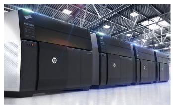
Already employed by manufacturers GKN Powder Metallurgy and Parmatech for the factory production of final parts, the Metal Jet printer combines years of HP printhead and chemical know-how in a "groundbreaking, voxel-level binder jetting technology." The printer has a 430 x 320 x 200mm bed, and promises x4 the nozzle redundancy and x2 the printbars compared to other metal 3D printing solutions.
