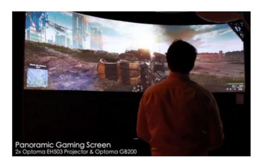
An edge-blended arch, 4.5m high and 8m wide, hung above the Optoma stand at ISE 2014.
