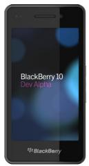
BlackBerry 10 is a shift from earlier versions, being an entirely new platform with a focus on virtual keyboards. The prototype device seen at Blackberry World has no physical keyboard-- it is a 4.2" iPhone-style device lacking in physical buttons.
