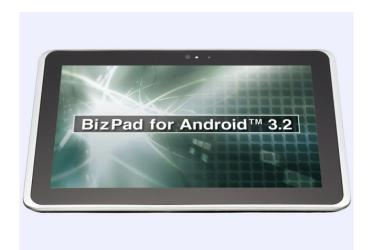
The tablets are shock-, dust- and water-proof, with a rugged form factor Panasonic claims withstands drops of up to 80cm (in the case of the 10" model) or 120cm (the 7").
