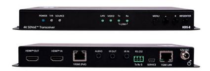
The transceiver is a fully standard and compliant SDVoE codec, and enables compatibility with other software and hardware streaming platforms. Being a transceiver, the KDS-8 can be set as either an encoder or decoder. As a decoder, it encodes and sends the HDMI input along with IR, RS-232 and analog audio over an IP network.
