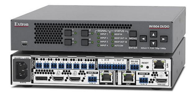
To ensure best-in-class image quality the switcher incorporates the Extron-exclusive Vector 4K scaling engine with 4:4:4 chroma sampling and 30-bit internal video processing. A DTP2 input and DTP2 output allow for easy AV and control signal extension up to 100m per endpoint over a shielded CATx cable.
