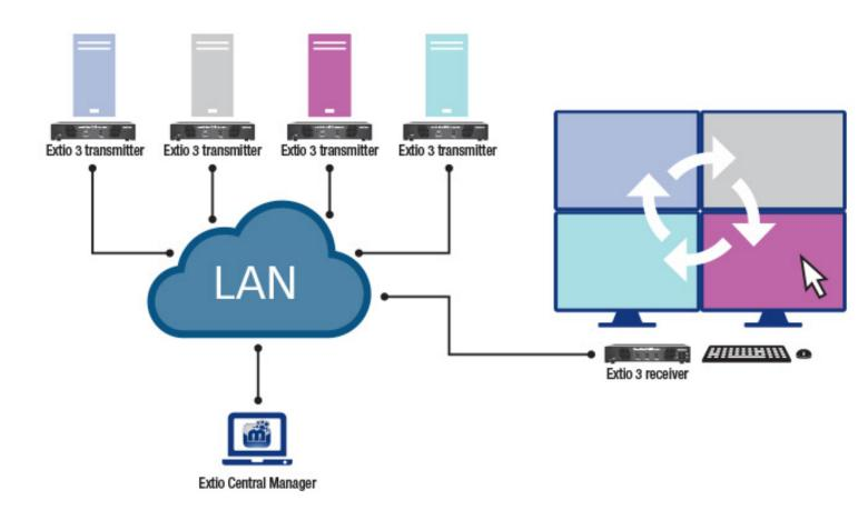
According to Matrox, Aggregator Mode streamlines operations by providing a unified view of information coming from different systems. Users can define which desktop gets mapped to
