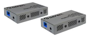
The EXT-DP-4K600-1SC extends HDCP 2.2, HDCP 1.4 and DPCP compliant DisplayPort 600MHz 4K audio/video over fibre. It supports WQUXGA (3840×2400), 4K Ultra HD (3840×2160), and 4K Cinema — DCI (4096×2160), up to 60 Hz frame rate and 4:4:4 Chroma sub-sampling. The AV signal is extended up to 200m, over a single strand of SC-terminated 50/125µm OM3 or better multi-mode fibre-optic cable.
