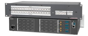
The 16x16 and 16x8 switchers are HDCP compliant and support 10.2Gbps data rates, Deep Colour up to 12-bit, 3D and HD lossless audio formats. Extron technologies such as SpeedSwitch, Key Minder and EDID Minder, together with automatic input cable equalisation and output relocking, ensure dependable operation with "exceptional" switching speeds and device compatibility.
