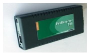
As the company puts it, fax machines are secure (since it is difficult to intercept faxes over analog phone lines), and as such remain popular with businesses. The ModuLAN digital fax receiver adds further security by converting faxes into PDF attachments emailed to intend recipients, thus further eliminating the risk of fax loss or interception, as well as the need for scanning or opting for digital storage.
