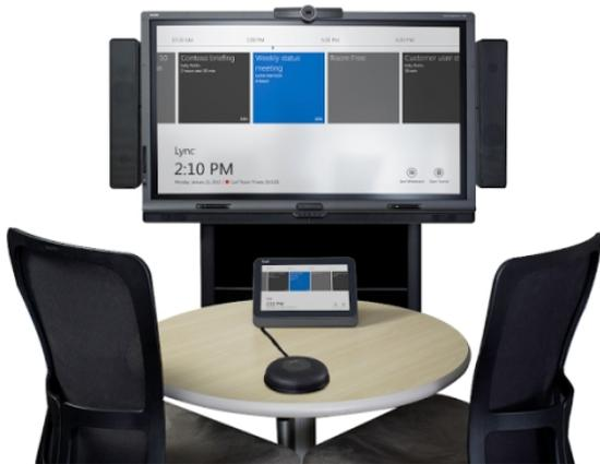
The system combines one or more interactive displays, wide-angle camera, customised speakers and microphones, and a room control console complete with 11.6-inch display. Each component is SMART-made, allowing for seamless integration and what the company describes as a "consistently rich meeting experience."
