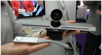
Yealink presents a 2nd generation videoconferencing solution aimed at huddle room use at ISE 2018-- the VC200, an all-in-one solution featuring camera and codec in a slim design customers can mount on top of monitors or TVs.
