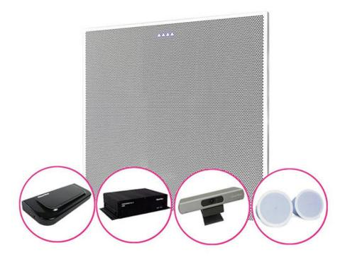
The BMA CTH performs acoustic echo cancellation, noise cancellation and beam selection, meaning no external DSP mixer is required. Adaptive steering (think of it as smart switching) provides "impeccable" room coverage. Also found built-in the BMA CTH are two 10W power amps driving the included 8-inch ceiling speakers.
