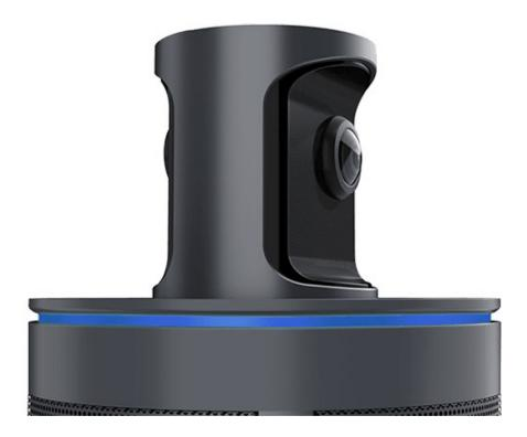
The camera captures all meeting attendees at 8K resolution, and is able to automatically focus on people as they speak. To locate the speaker and pickup their gestures and facial expression the camera uses Al-enabled facial recognition and eight omnidirection microphones to pick on the sound. Remote participants on the other end get a 1080p resolution stream with closeups on the speakers, making them feel like everyone is in the same room.
