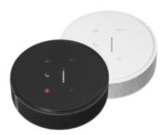
The top features a capacitive touch control surface, meaning button-free operation and no "clicking" noises on the other side. Vaddio says it should cover most meeting rooms, thanks to full 360-degree coverage via 3 unidirectional condenser microphone elements. Each of the unidirectional cardioid microphone elements is equipped with integrated echo cancellation and Digital Signal Processing (DSP), including equalisation, filtering and automatic gain control (AGC).
