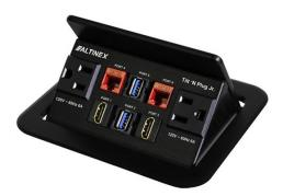
Users can access inputs by pushing down on the top cover, allowing the unit to tilt open. Pressing on the top cover until the latching mechanism engages hides the inputs. In closed position the top panel lies nearly flush with the tabletop, held in place by the latching mechanism.
