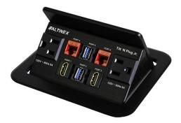
Users can access inputs by pushing down on the top cover, allowing the unit to tilt open. Pressing on the top cover until the latching mechanism engages hides the inputs. In closed position the top panel lies nearly flush with the tabletop, held in place by the latching mechanism.
