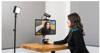
To turn on the system, one simply inserts a USB stick and presses the record button to start recording. The system powers up automatically, and once the recording is complete, removing the USB storage puts it back in standby mode and turns off any devices connected to the power controller. The core components fit securely in an equipment rack, with only the control panel and USB connection visible to the user.
