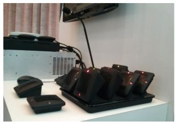
The Executive Elite uses distributed architecture to connect a remote antenna receiver and base DSP units via standard Cat 6 cable complete with Power over Ethernet (PoE). Such a system improves wireless connectivity by allowing the placement of recievers and wireless microphones in the same room.
