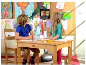
The Beam+ looks like a 10-inch iPad on top a 3-wheel motorised mount, and features two 640x480 HDR cameras, 4-microphone array and a "powerful" amplifier. Once connected to the internet it allows users to maneuver around the house in real-time and check what the kids, pets or friends are getting up to while video chatting via included software.
