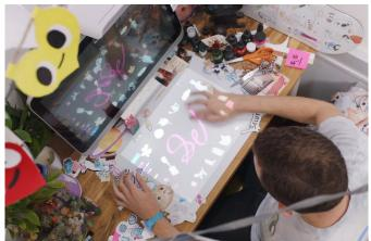
From a distance the Sprout looks like an All-in-One PC, only the keyboard is replaced by a mat and what looks like an desk lamp hangs on top of a 23-inch touchscreen. However the "mat" is actually a capacitative touch surface, and the "desk lamp" combines an Intel RealSense 3D camera, 14.6MP camera and a DLP projector beaming a work surface on the mat.
