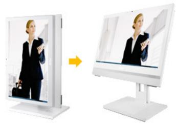
The AP16 is a 16" mode with x2 built-in COM ports (making it ideal for cash registers or barcode readers), while the AP2011 is 20" in size. The AP16 supports fast boot from USB stick (allowing users to quickly switch between operating systems) while the AP 2011 features an adjustable stand and carries a second-generation Intel Core processor.
