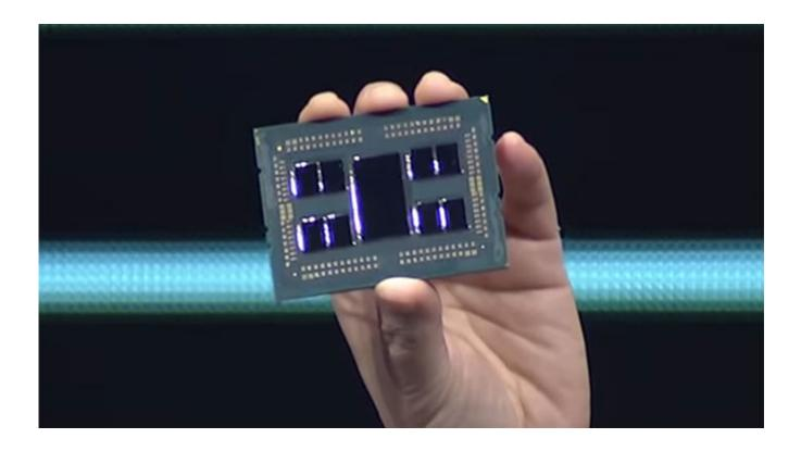
Described as nothing less than "one CPU to rule them all in 2020," the Threadripper 3990X is essentially a consumer version of the Epyc 7702P server processor. As the first 64-core high-end desktop processor, it offers 128 threads of processing power and clock speeds reaching 2.9GHz with a boost of up to 4.3GHz. As such, it is aimed less at regular customers and more at professionals working on video editing and 3D rendering.
