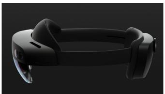
As an upgrade on the first Microsoft headset, the HoloLens 2 offers double the field of view even as it maintains the same 47 pixels per degree of sight. The company does not give exact numbers on the matter, instead saying it is the equivalent of moving from a 720p TV to a 2K set for each eye. The headset tracks the retinas to work out what the user is looking at, and uses a new "time-of-flight" depth sensor to track the hands without need for a controller.
