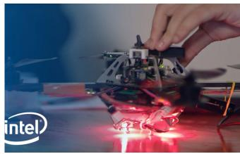
The Aero is a full-assembled drone complete with integrated flight controller, remote control receiver and transmitter. Since it is an Chipzilla product it uses an Intel CPU (specifically an Atom x7-Z8750) and a 3D RealSense depth camera, which come in handy when used together with GPS, altimeter and magnetometer to power an auto-pilot mode.
