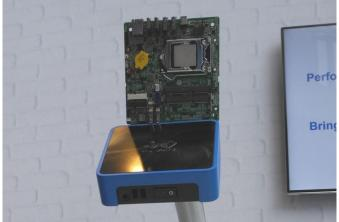
Named after their dimensions (5.5- x 5.8-inch, or 140 x 147mm), 5x5 motherboards have a 29% smaller surface area than the mini-ITX standard. The boards build on Intel's NUC mini-PC concept, and feature a land grid array (LGA) processor socket, two laptop-style SODIMM slots and storage in either 2.5-inch SATA or M.2 SSD form.
