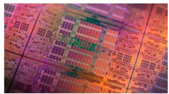
The 9500-series processor carries Intel Itanium Architecture (IA64 ISA) and packs 3.1 billion transistor into a 32nm die. It also doubles core count (8 from 4), carries up to 54MP of on-die memory and enables up to 2TB of low-voltage DIMMs in a 4-socket configuration.
