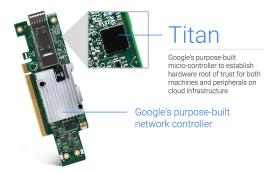
As the blog post explains, the Titan chip integrates with the secure boot process. This involves the server boot a known firmware/software stack, cryptographically verify the stack and then gain (or fail to gain) access to network resources according to the verification. Titan also adds further layers of security, namely remediation (reestablishes trust in the event of firmware bugs) and first-instruction integrity (identifies the earliest code running on each machine's startup cycle).
