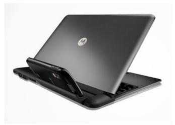
What makes the Android 2.2 set unique are the 2 docks, which can turn the smartphone into either a mobile PC (the dock connects to a display, keyboard and mouse) or a laptop (complete with 11.6" screen).
