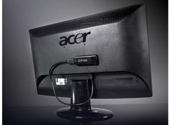
The Ceptor features a configurable, persistent and fully manageable enterprise client desktop, making it ideal for a variety of applications. Handling virtual desktop access is ZeTOS, the Devon IT zero client OS.
