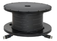
The cables are HDCP 1.4/2.2 compliant, and support resolutions up to 8K/30Hz (4:4:4) for cable lengths up to 50m, and 4K/60Hz (4:4:4) for lengths reaching up to 100m. Construction features a hybrid design consisting of four POF (Polyflourinated Optical Fibre) and six copper wires.
