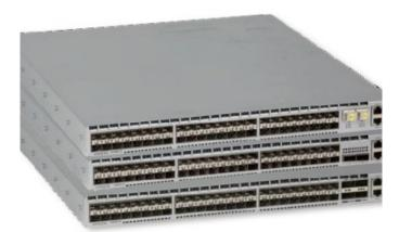
The company's so-called "leaf" switches are data centre switches handling traffic flow between servers. With the 100GbE uplink ports Arista says the switches offer a 1000x increase in packet memory compared to typical switches in top-of-rack applications.
