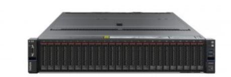
The two servers support up to 128 cores, together with up to 4TB of DDR4 memory. Lenovo adds the adoption of PCIe 4.0 technology delivers double the I/O bandwidth of previous-generation servers, eliminating potential bottlenecks and increasing network capabilities. The company adds the servers are ideal for financial services, retail and manufacturing applications, as well as customers wanting to run performance-sensitive workloads at higher speeds with lower total cost of ownership.
