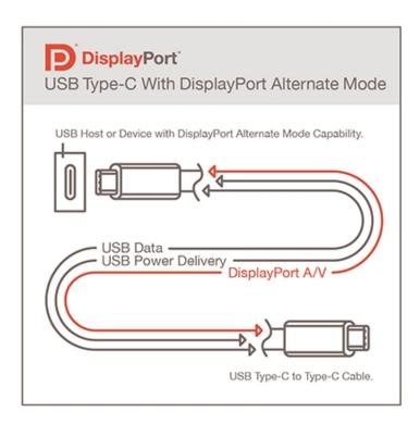
DisplayPort Alt Mode 2.0 fully enables all the features of the latest version of the DisplayPort standard (version 2.0) through the USB-C connector. Through Alt Mode, the USB-C connector can transmit up to 80Gbps of DisplayPort video data utilising all four high-speed lanes in the cables, or up to 40Gbps with simultaneous SuperSpeed USB data delivery.
