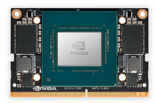
The Jetson Xavier NX measures 45 x 70mm, making it around the size of a credit card. It is based on the same Xavier SoC as the Jetson AGX Xavier, and and as such has the same Volta GPU and NVDLA accelerator cores. Nvidia says it delivers "server-class" performance of up to 21 TOPS, allowing it to run AI workloads while consuming 15W of power. For lower power consumption it can clock up to 14 TOPS at 10W.
