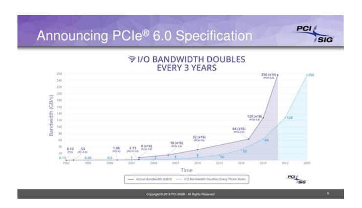
The organisation completed the PCIe 5.0 specification just a few months ago, specifically on May 2019. We know little as to how version 6.0 will improve on it, other than the doubling of the data rate to 64 GT/s while maintaining backward compatibility with all previous spec generations. For the curious, the 64 GT/s figure refers to GigaTransfers per second over the interface, and clocks to around 256GB/s of bandwidth (or 128GB/s in each direction).
