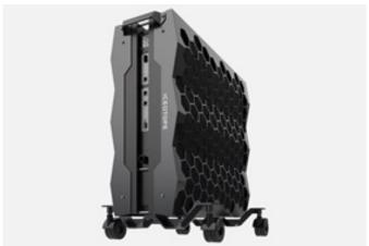
Usable as either a workstation or a micro datacentre, the EdgeStation is a sealed liquid cooling system. The electronics are immersed in dielectric fluid, making a virtually silent system with no fans or other air cooling equipment. The casing is IP54-rated for resistance to extreme heat, humidity and dust, while built-in wheels make it portable.
