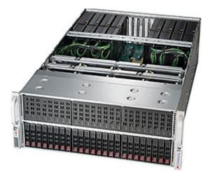
The platform behind the Nvidia Iray Visual Computing Application (VCA), the SuperServer features airflow-optimised architecture with independent cooling zones and a side-by-side component layout. According to the company this eliminates CPU/GPU preheat, enabling maximum performance from eight 300W GPUs and two 150W CPUs.
