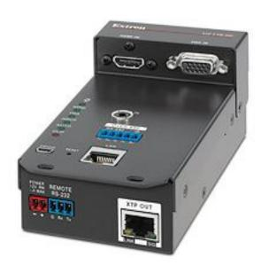
Extron Electronics introduces the **XTP T FB 202**, a two-input XTP transmitter in a unique form factor designed for floor boxes commonly used in European AV installations.
