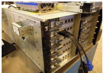
Similar to other x86-based microservers such as HP Moonshot, NeXtScale is a minimalist, dense server design using half-width server nodes. Designed to eventually replace the iDataPlex line, the system incorporates up to 86 systems and 2016 processing cores within a 19-inch rack.
