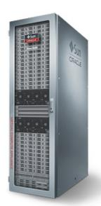
The Virtual Compute Appliance ships fully assembled and is based on the Oracle X3-2 servers. It includes two 8-core Intel Sandy Bridge-EP Xeon E5 processors running at 2.2GHz.
