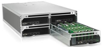
The launch follows 18 months of development since the November 2011 announcement of Project Moonshot. It was first revealed as "Redstone," an ARM-based design packing either 288 EnergyCards (a Calxeda reference design packing x4 EnergyCore SoCs, x4 DIMM slots and x4 SATA slots on a single daughterboard) on a 4U rack-mount server or 2800 on a full rack, together with shared power, cooling and management infrastructure.
