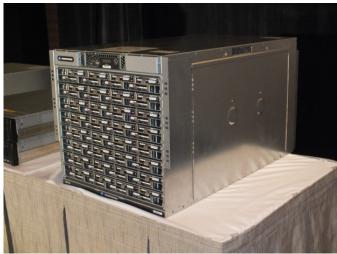
The SM15000 uses SeaMicro's Feedom Fabric to build "micro" servers, allowing data centres to expand compute, networking and storage capacities independently.
