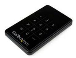
Windows, Mac and Linux compatible, the enclosure supports 2.5" SATA HDDs and SSDs (up to 9.5mm in height) and offers real time 256-bit AES hardware encryption via high-speed 32-bit ARM-based controller. The built-in touchpad simplifies password entry while providing access to encrypted content.
