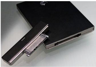
Part of the SATA 3.2 Revision, USM Slim trims the port to 9mm (down from 14.5mm) in order to allow integration with thinner devices.
