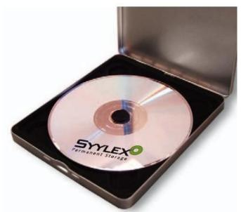
The discs consist of 2 halves-- an engraved durable glass substrate (made from glass the chemical industry uses to store aggressive reagents) and a metallic alloy reflective layer. The 2 halves are bonded together, and metal and bond are in turn nearly entirely enclosed in glass.
