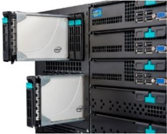
The SSD 710 uses compute-quality 25nm MLC flash memory with Intel High Endurance Technology (HET), unlike the Single-Level Cell (SLC) using X25-E.
